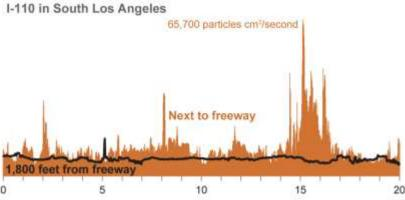
Source: TSI P-Trak Ultrafine Particle Counter 8525 readings on Aug. 20, 2015 and Sept. 24, 2015. See the data
